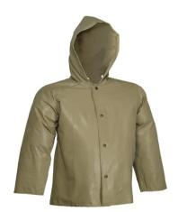
**Compliance Standards:** Flame resistant. Self extinguishing with flameout and afterglow less than or equal to 2 seconds after removal of ignition source and char length of less than 6 inches. Test Method ASTM D6413.
